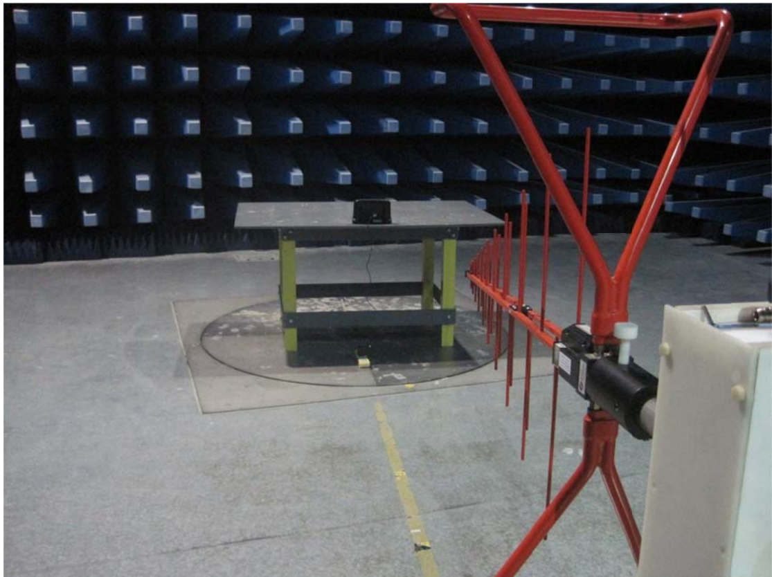
Radiated Spurious Emissions Test Setup (30MHz-1GHz)
