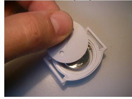
5. Screw cap on clockwise until it stops and cap is level with transmitter case bottom
