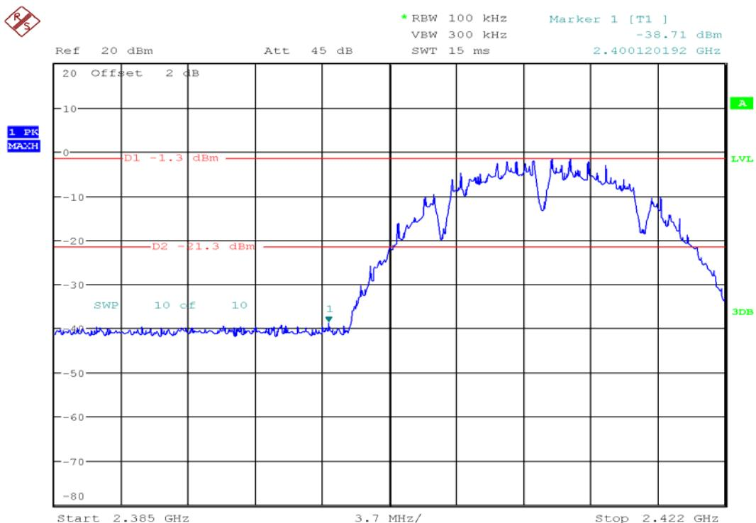
2) Out of band emissions & Band edge(Radiated)
