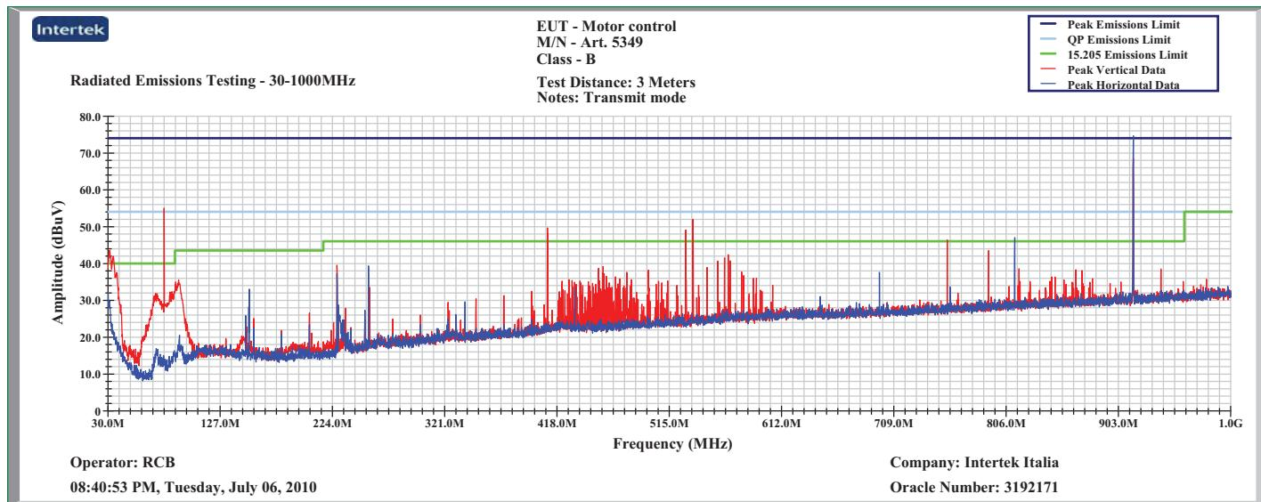
Transmit mode - radiated emissions from 30-1000MHz
