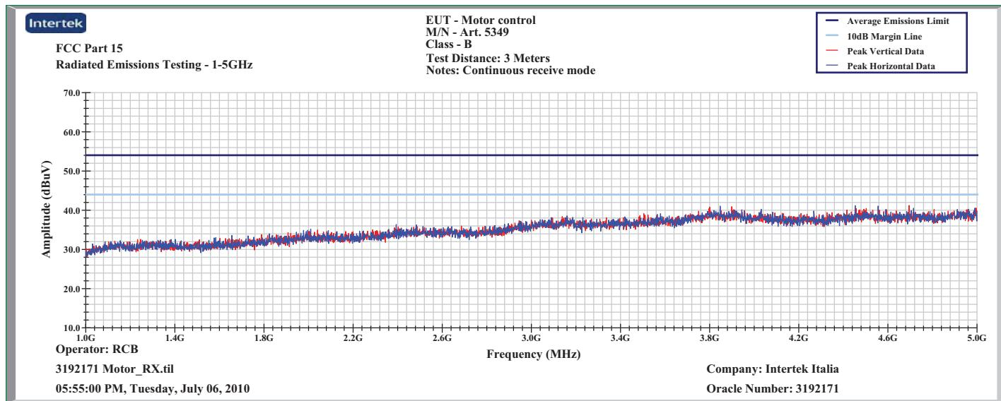
Receive mode - radiated emissions from 1-5GHz
