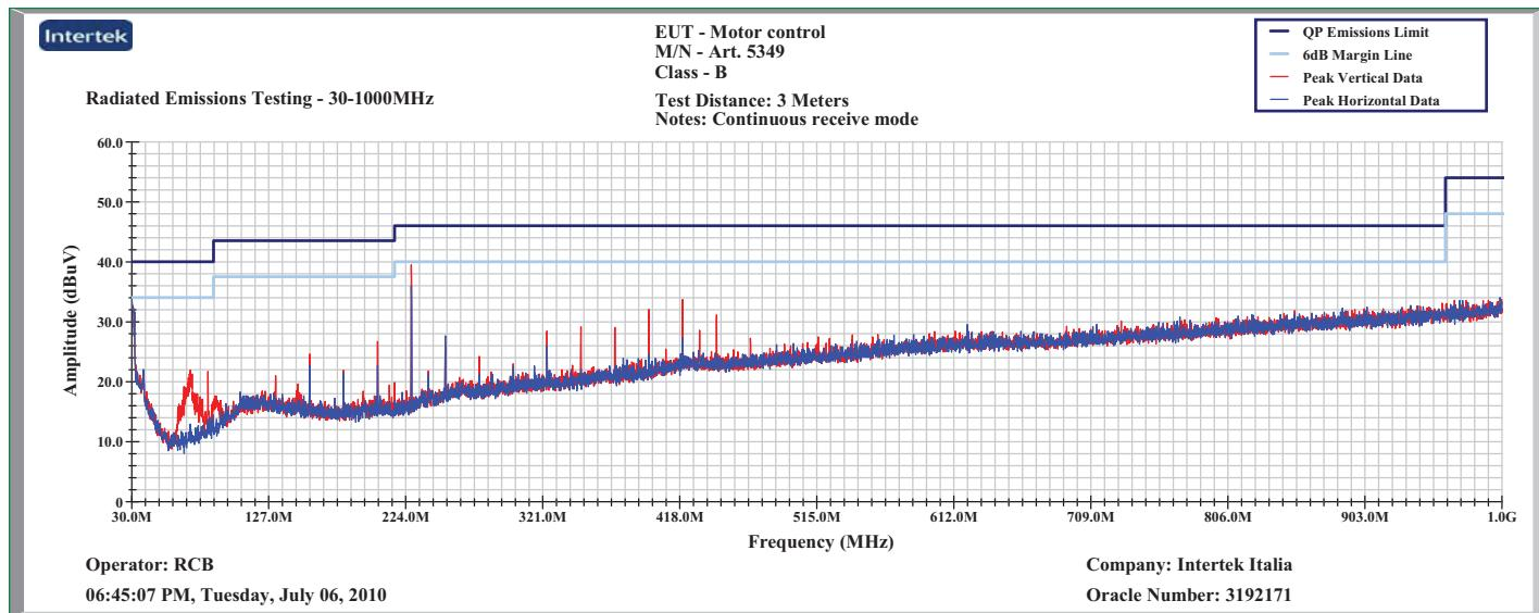
Receive mode - radiated emissions from 30-1000MHz
