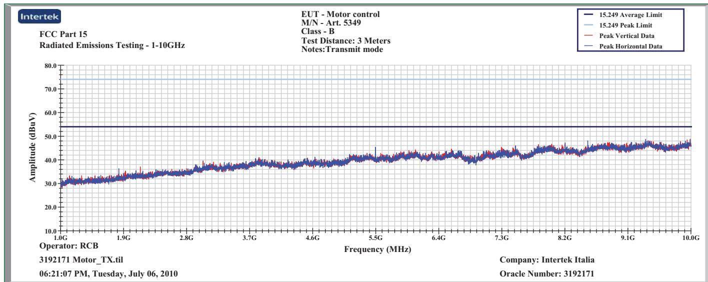
Transmit mode radiated emissions from 1-10GHz
