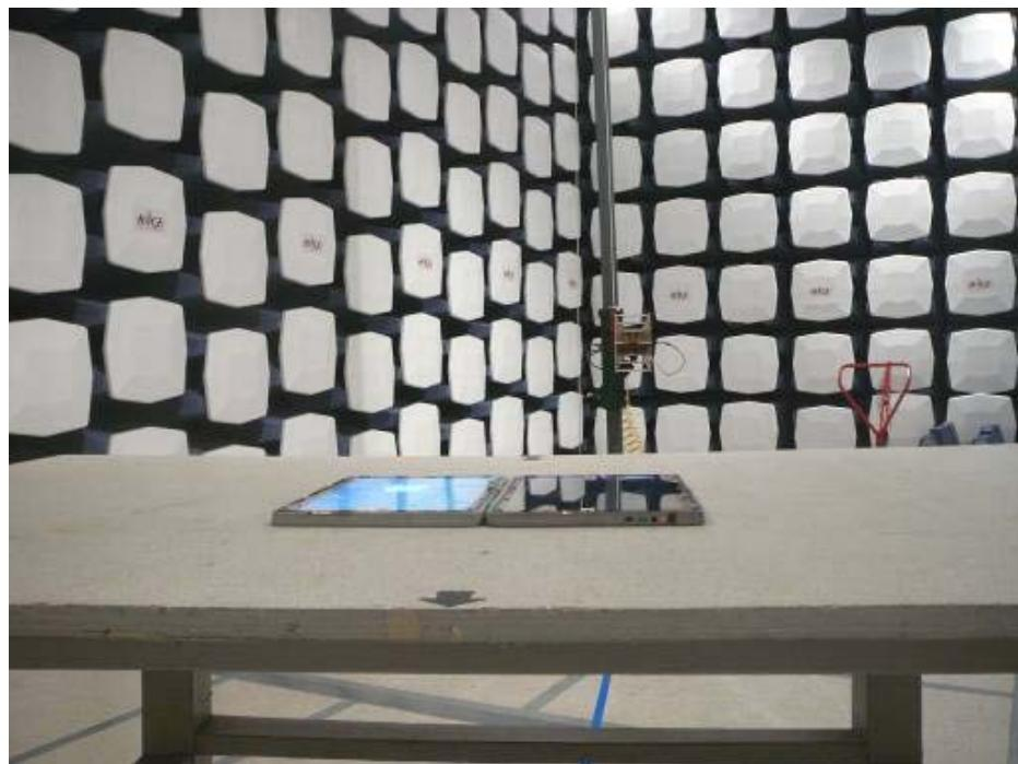
**10.5 AC Line Conducted Emission Front View**
