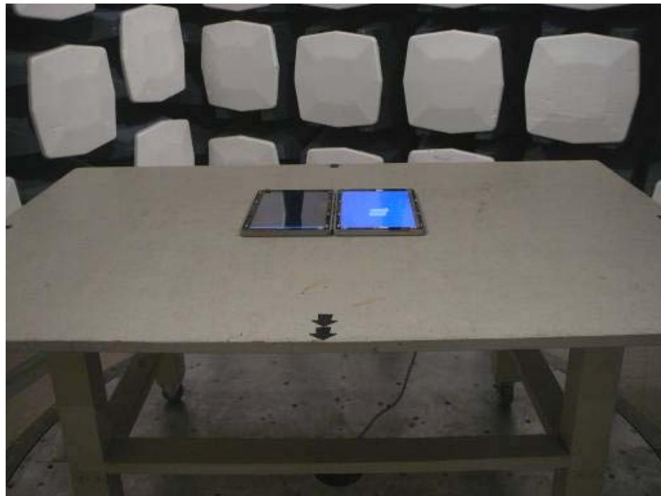
**10.4 Radiated Emission above 1 GHz Rear View @ 3 Meter**
