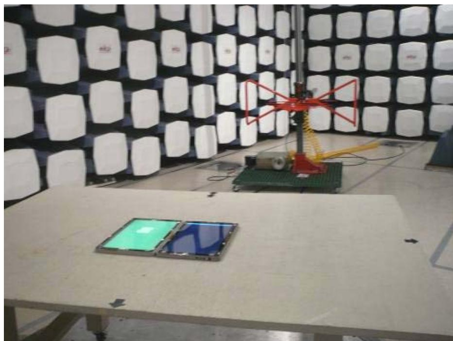
**10.3 Radiated Emission above 1 GHz Front View @ 3 Meter**
