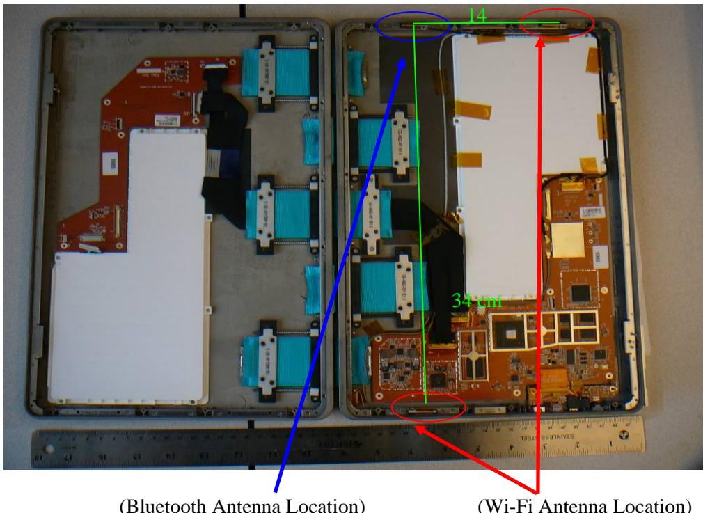
\*Note: One EUT with Wi-Fi antenna located at the top, and another EUT with Wi-Fi antenna located at the bottom; However, both antenna path controlled by the switch circuit as shown below, the unit auto pick the best sensitive antenna and do the transmit; two antenna can not be transmit as the same time only one or the other.
