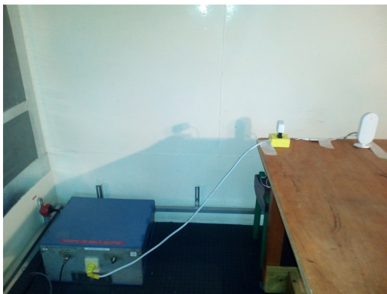
Photograph 8.1.1 Setup for conducted emission measurements
