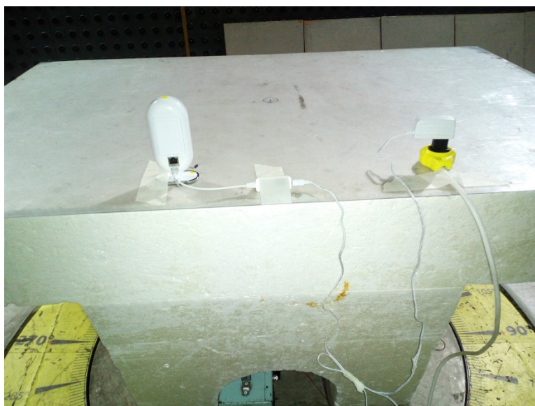
Photograph 8.2.3 Setup for radiated emission measurements, EUT cabling
