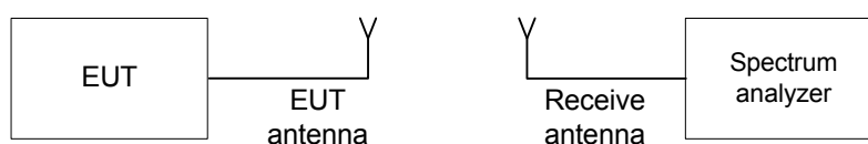
Figure 7.2.1 Occupied bandwidth test setup
