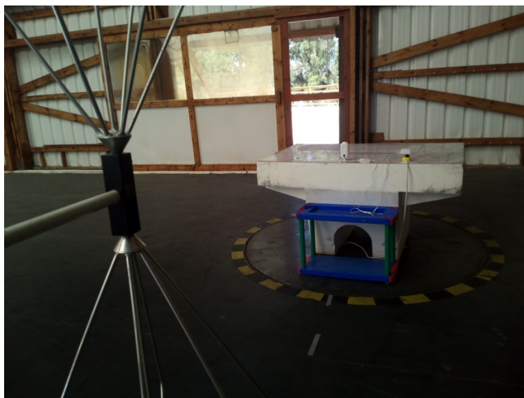
Photograph 8.2.3 Setup for radiated emission measurements, EUT cabling
