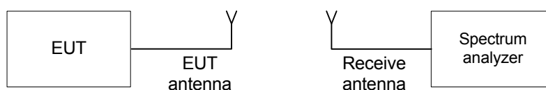
Figure 7.4.1 Occupied bandwidth test setup
