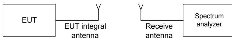
Figure 7.1.1 Setup for transmitter shut down test
