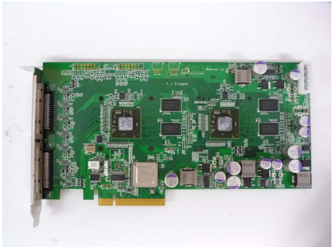
FIGURE 1 GRAPHIC CARD (M/N: FI5400E-2G8H1GF(8-HDMI)) MAIN BOARD HEAT SINK REMOVED
