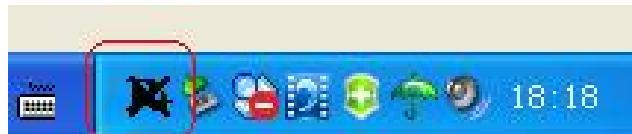
When an USB wireless adapter is inserted into an USB 2.0/1.1 port of Notebook or PC, the icon changes colors according to the wireless signal quality.
