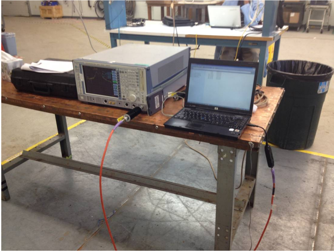
Antenna Port Conducted Test Setup
