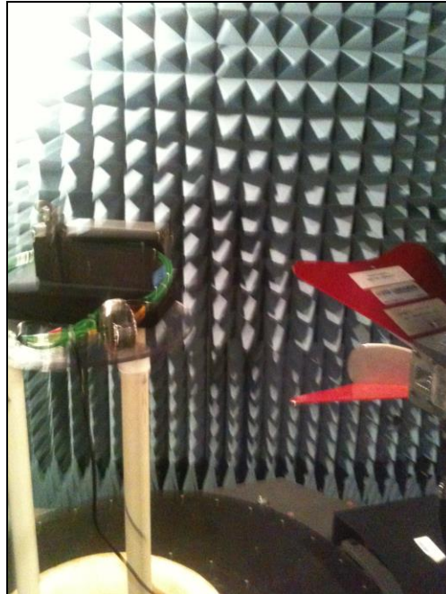
Photograph 4. Radiated Spurious Emissions, Test Setup, 1 GHz – 18 GHz
