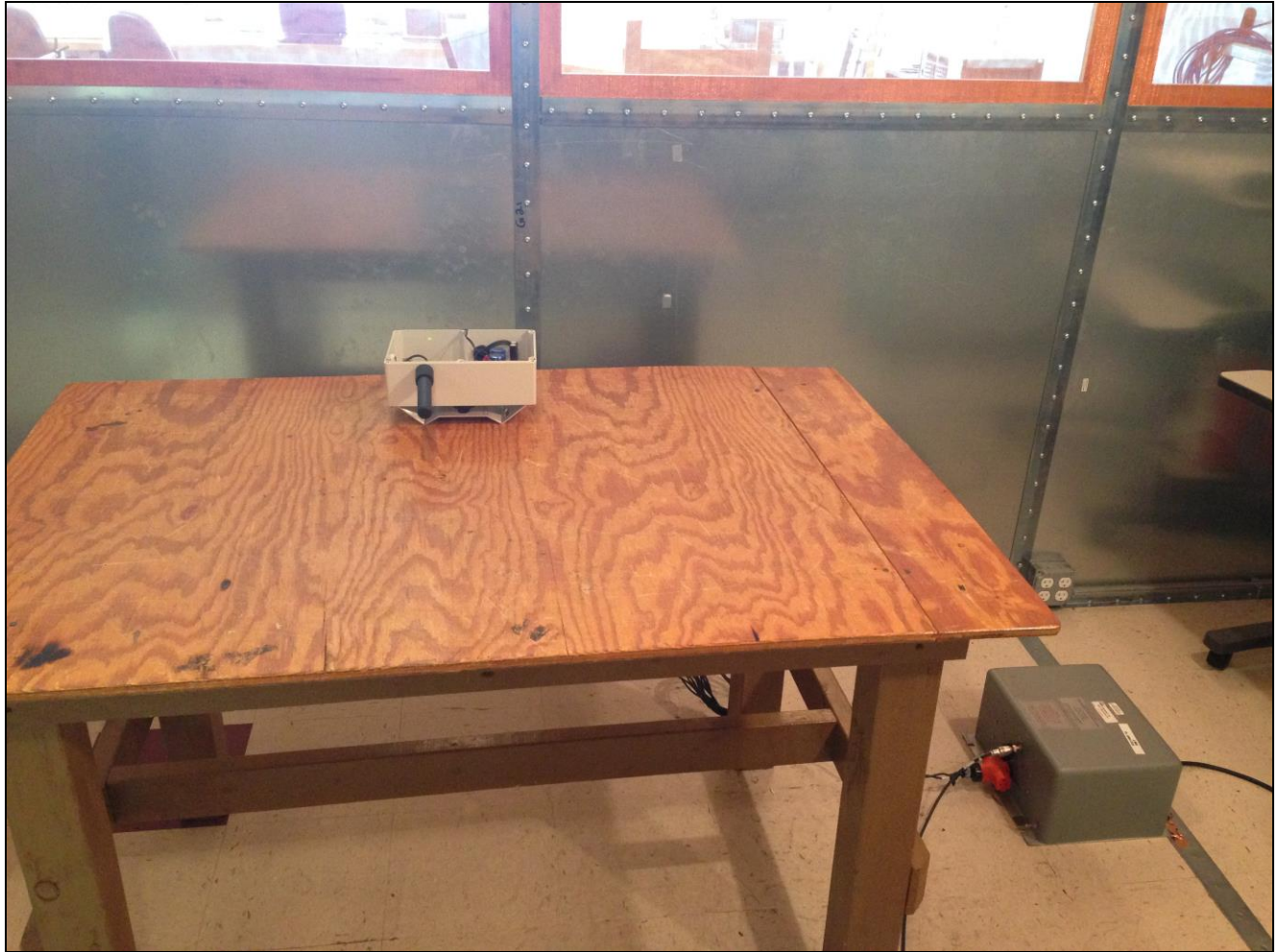
Photograph 1. Conducted Emissions, Test Setup
