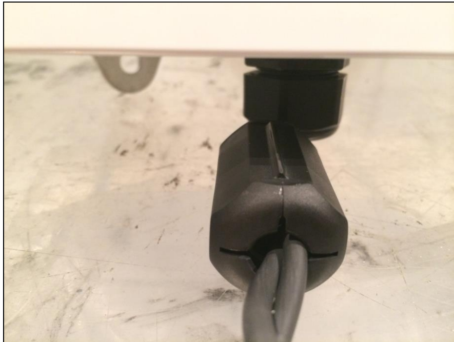
Photograph 4. Radiated Emissions, Test Setup, Ferrite on Unit
