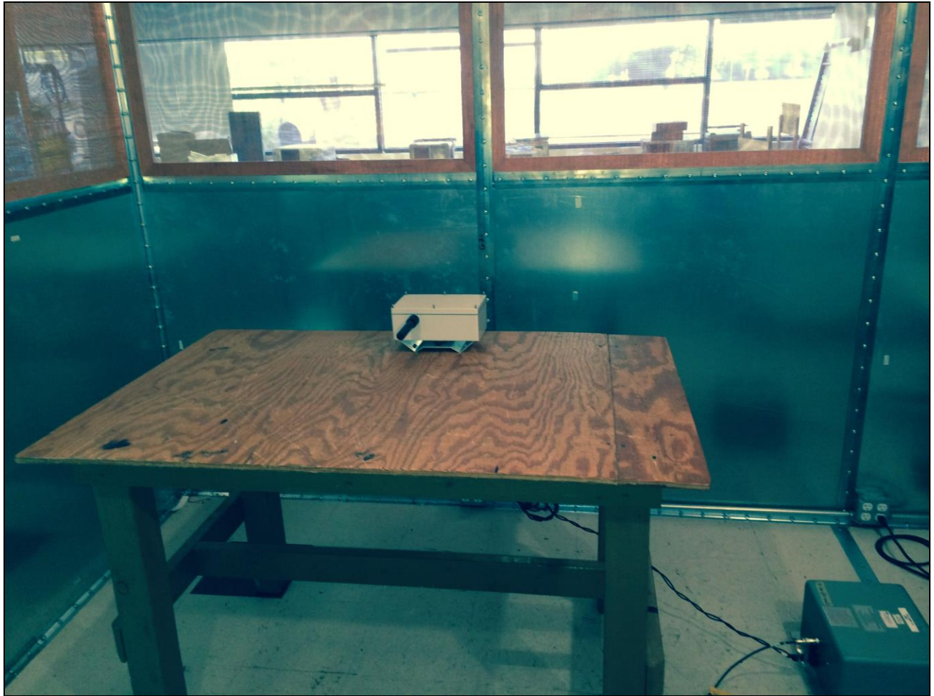
Photograph 5. Conducted Emissions, 15.207(a), Test Setup
