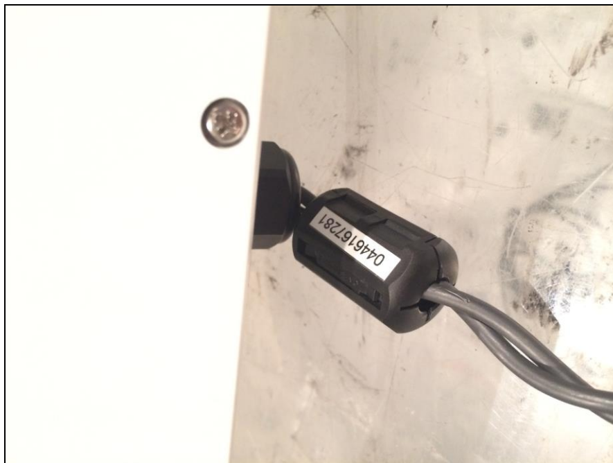
Photograph 3. Radiated Emissions, Test Setup, Ferrite Model Number
