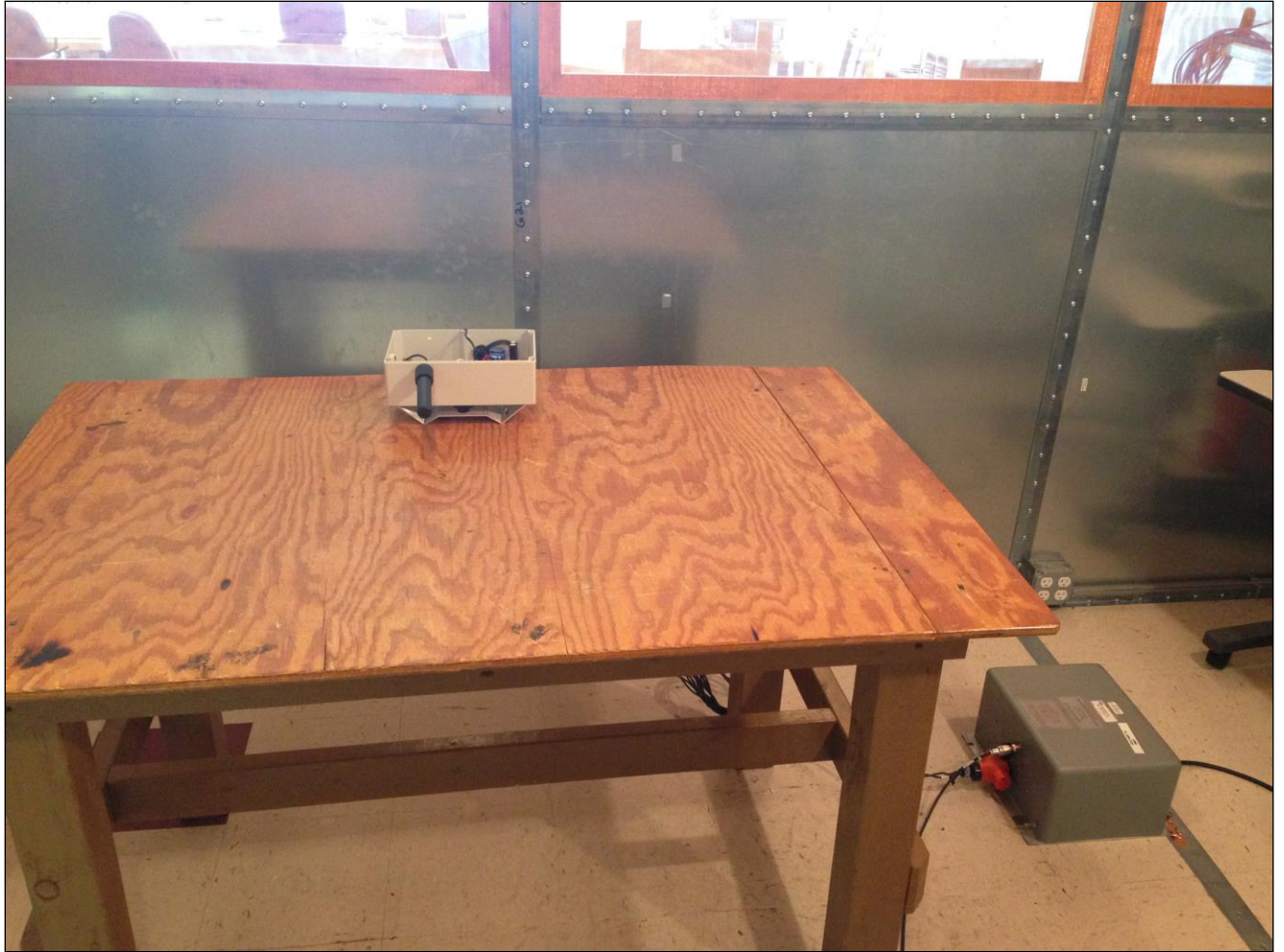
Photograph 1. Conducted Emissions, Test Setup
