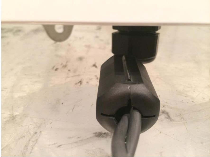
Photograph 4. Radiated Emissions, Test Setup, Ferrite on Unit
