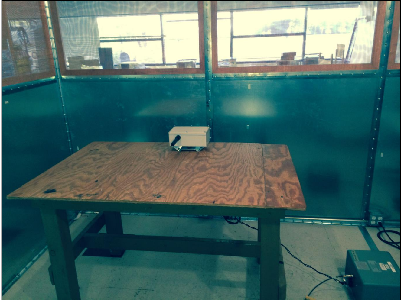
Photograph 5. Conducted Emissions, 15.207(a), Test Setup
