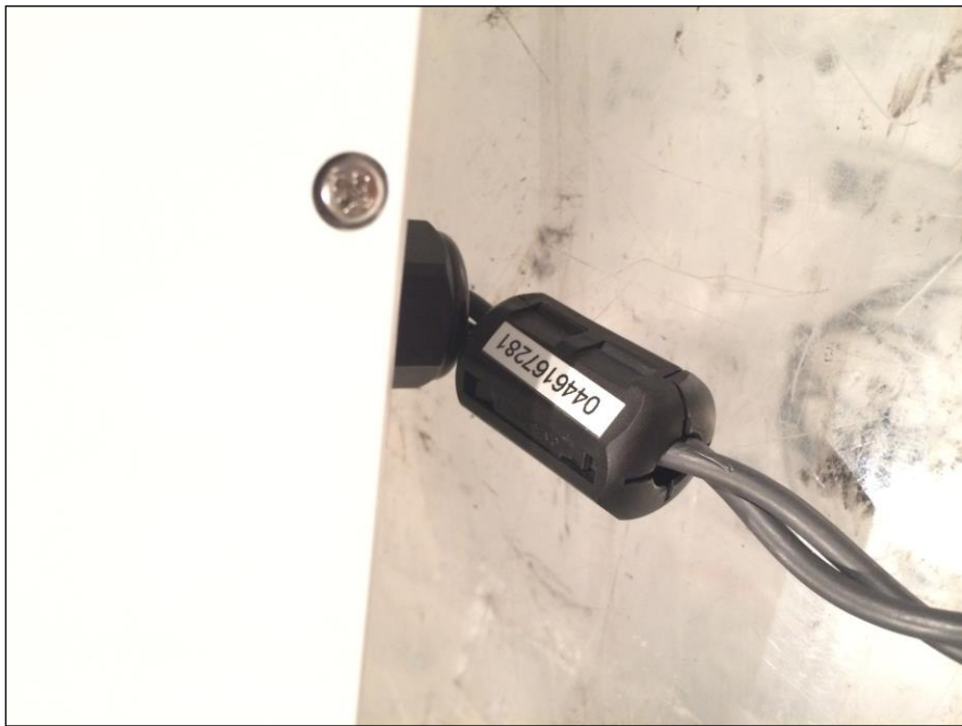
Photograph 3. Radiated Emissions, Test Setup, Ferrite Model Number
