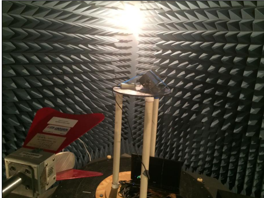
Photograph 3. Radiated Spurious Emissions, Test Setup, 1 GHz – 18 GHz
