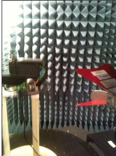
Photograph 4. Radiated Spurious Emissions, Test Setup, 1 GHz – 18 GHz
