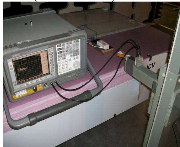
HF Harmonic Mixer (antenna/pre-amp/cables) (18 GHz to 26.5 GHz)
