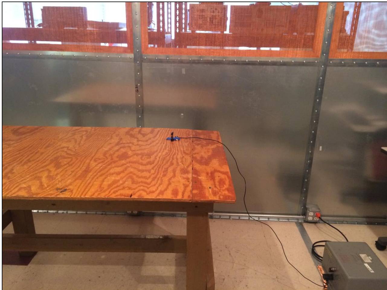
Photograph 1. Conducted Emissions, Test Setup
