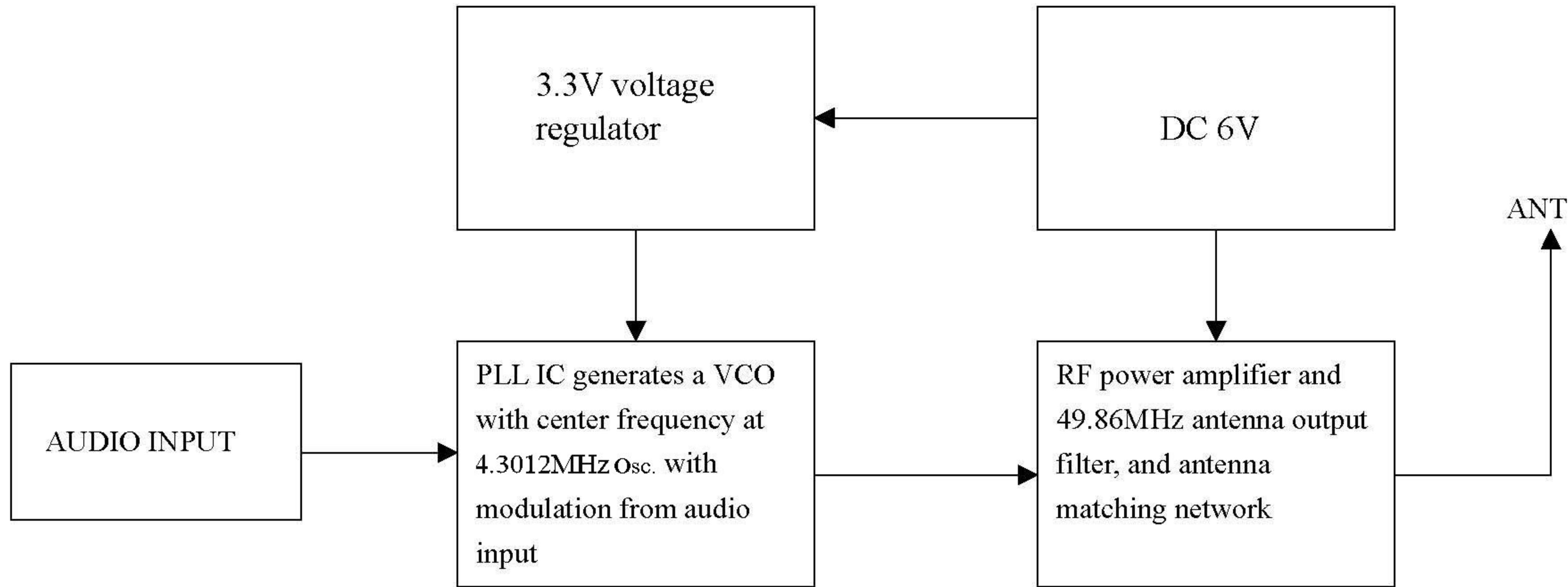
49.86MHz transmitter operation block diagram
