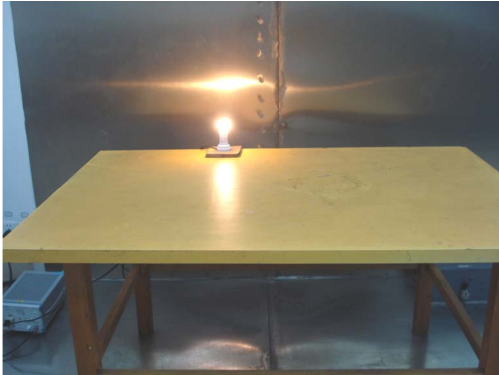
Conducted Emission Test Setup Front View
