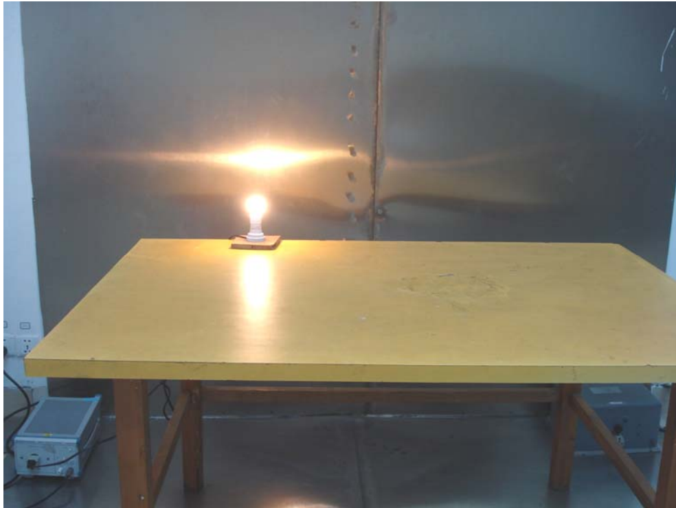
Conducted Emission Test Setup Front View
