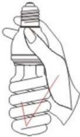
CORRECT WAY (JUST GRASP BASE PLASTIC PART)
