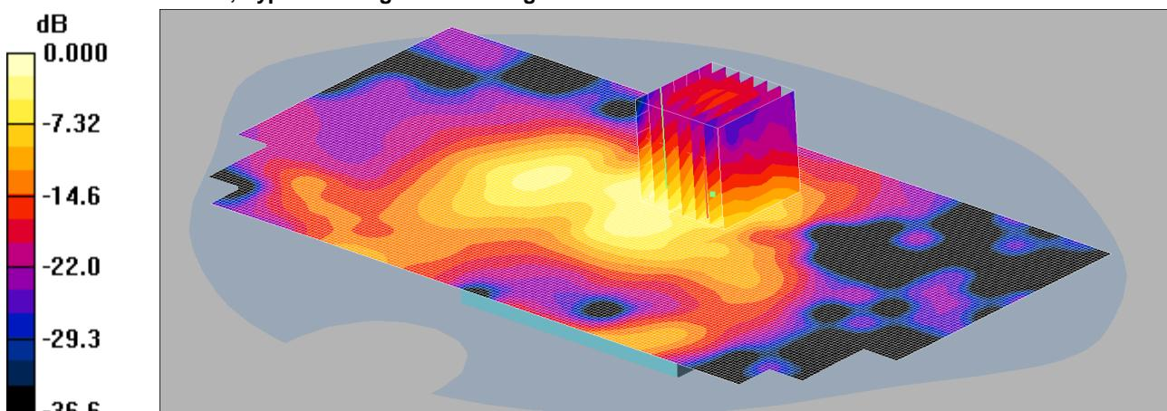
Communication System: WLAN; Frequency: 2437 MHz; Duty Cycle: 1:1
