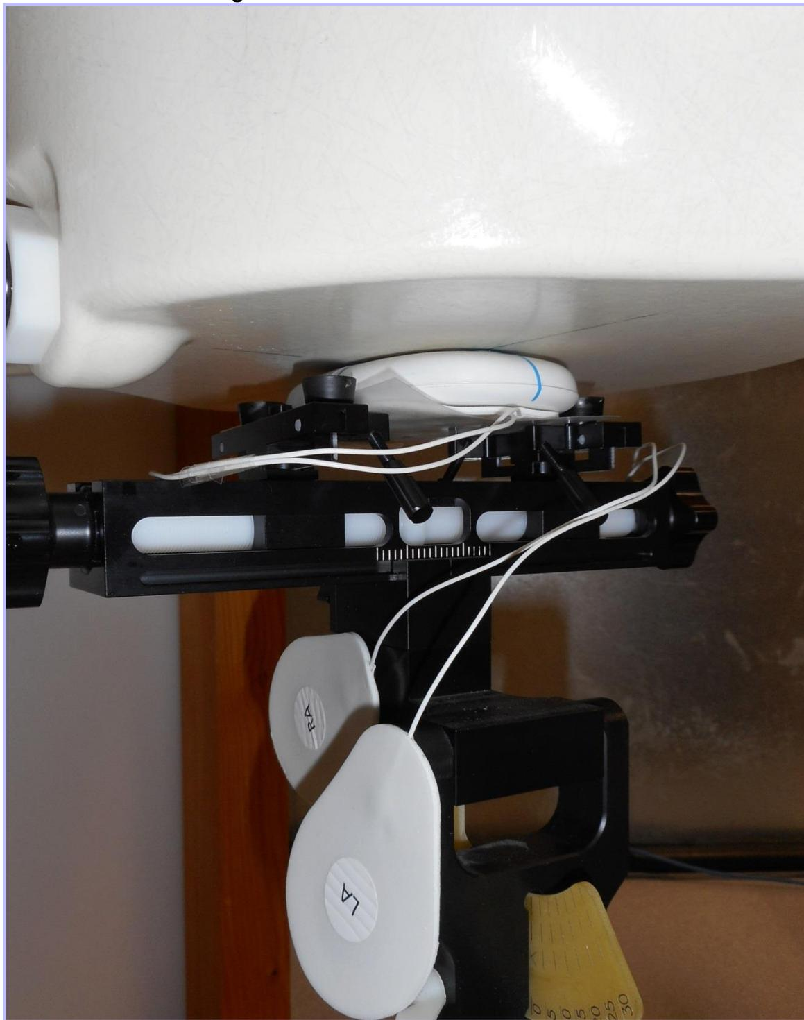
**004: Front of EUT Facing Phantom With Electrode Array Attached Within the Fluid Sandwich**
