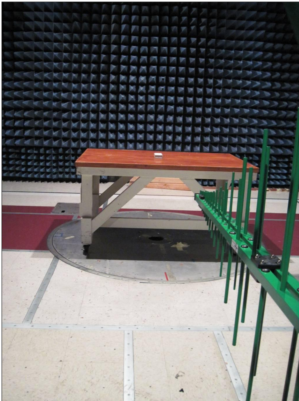
Photograph 2. Radiated Emission, Test Setup
