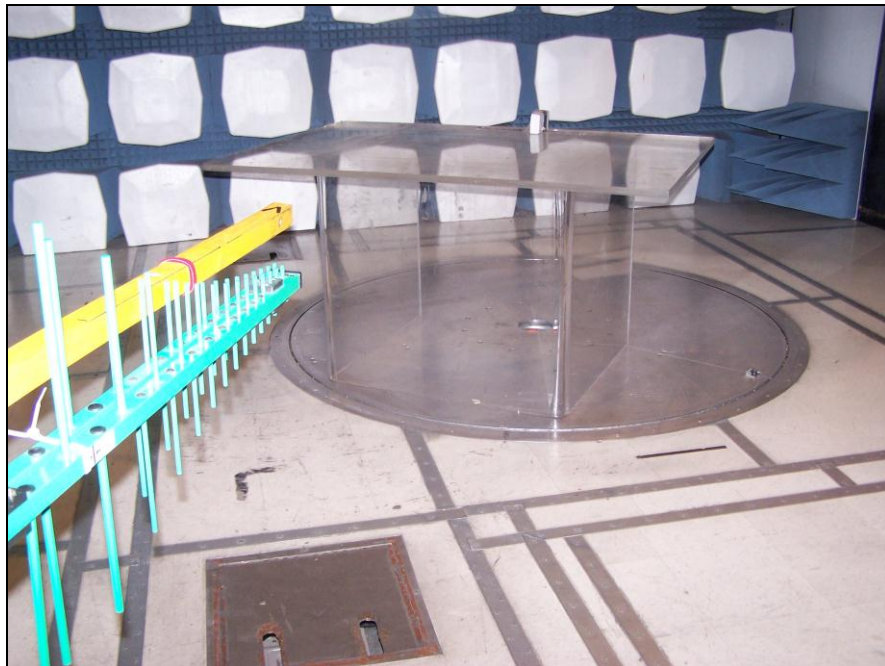
Photograph 4. Radiated Spurious Emissions, Test Setup 2
