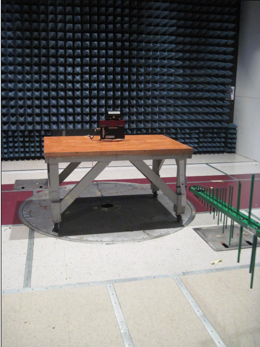
Photograph 1. Radiated Emission, Test Setup
