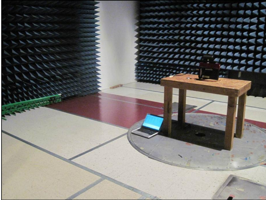
Photograph 2. Radiated Spurious Emissions, Test Setup
