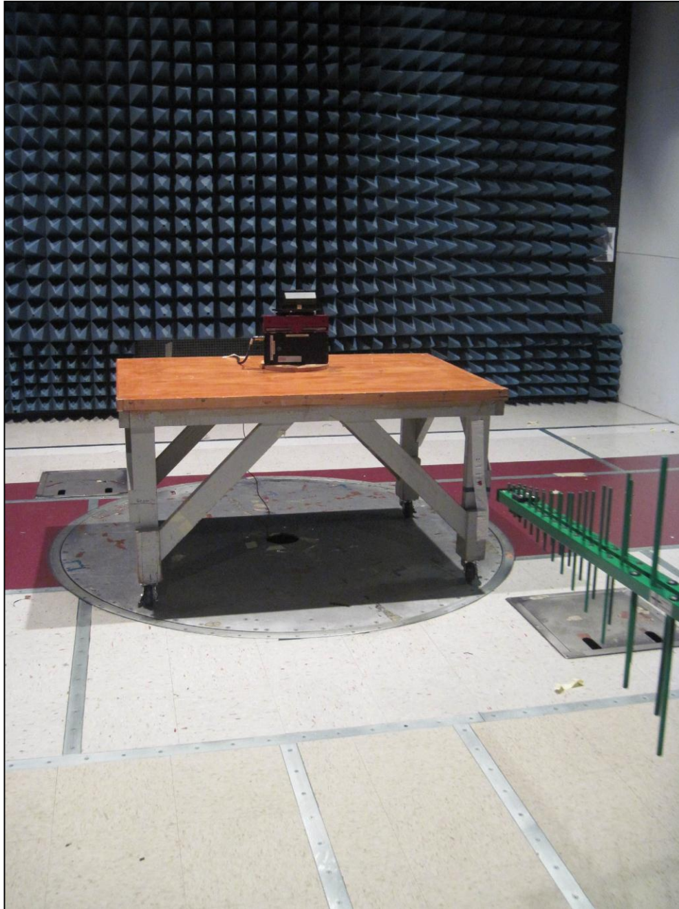
Photograph 2. Radiated Emission, Test Setup
