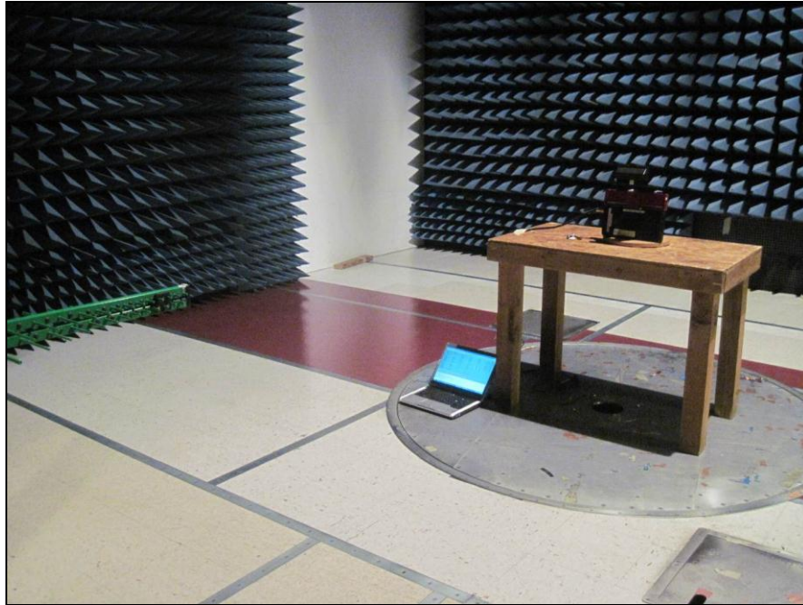
Photograph 3. Radiated Spurious Emissions, Test Setup
