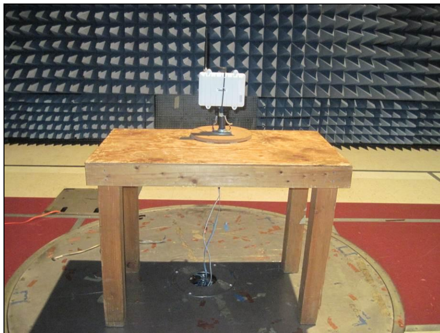
Photograph 4. Radiated Spurious Emissions, Test Setup
