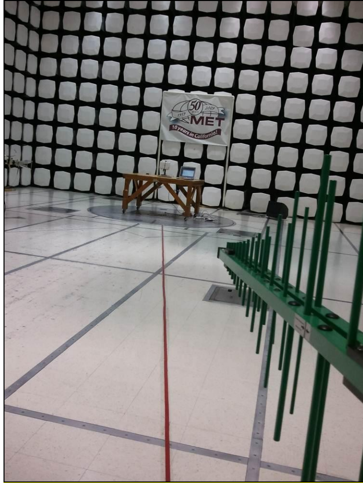
Photograph 2. Radiated Emission, Test Setup
