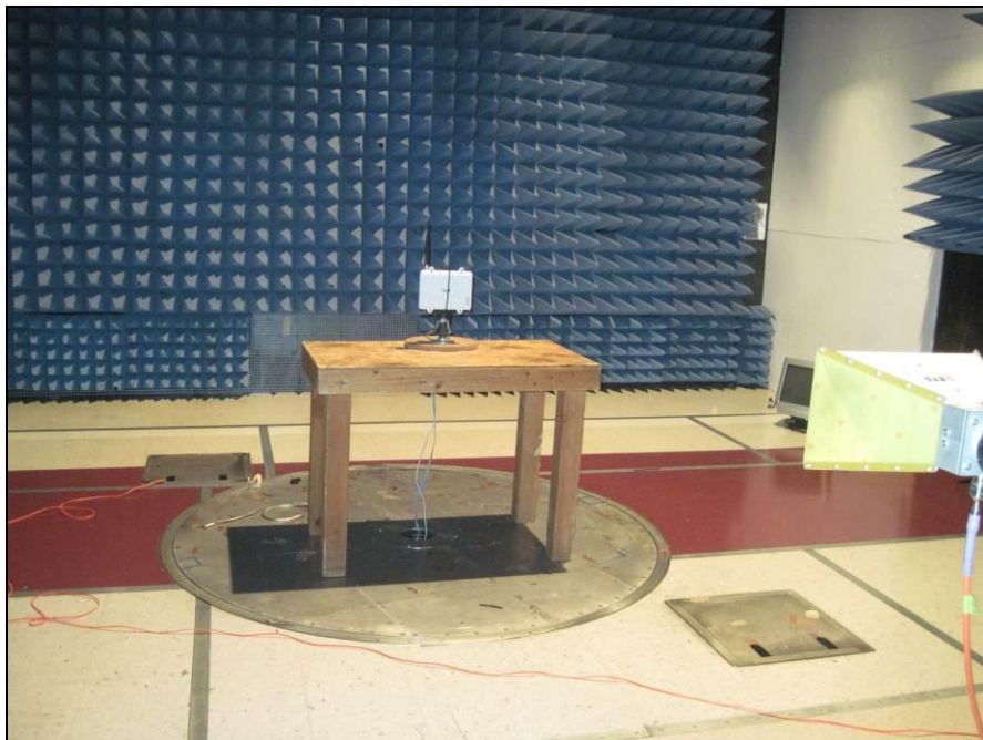
Photograph 6. Radiated Spurious Emissions, Test Setup, 1 GHz – 18 GHz
