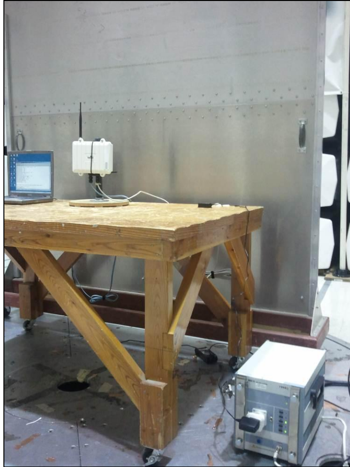
Photograph 3. Conducted Emissions, 15.207(a), Test Setup
