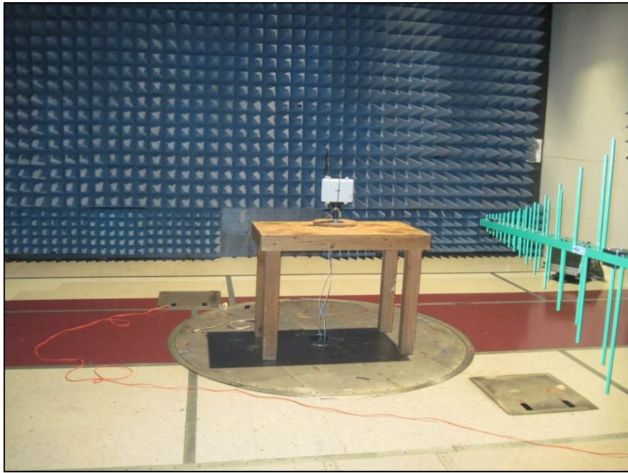
Photograph 5. Radiated Spurious Emissions, Test Setup, 30 MHz – 1 GHz
