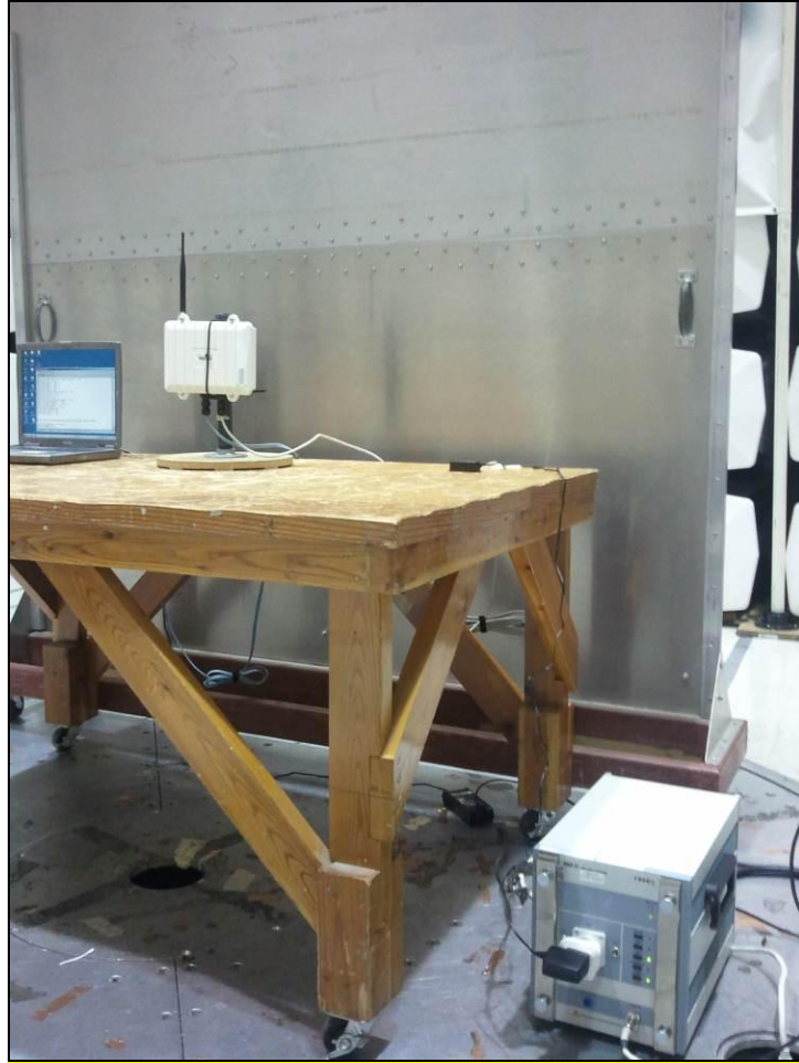
Photograph 1. Conducted Emissions, Test Setup
