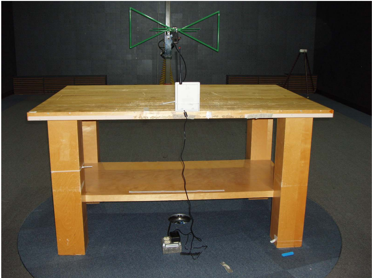
Photo 2 – Rear View of the Radiated Emissions Test Set-up 30 - 1000 MHz
