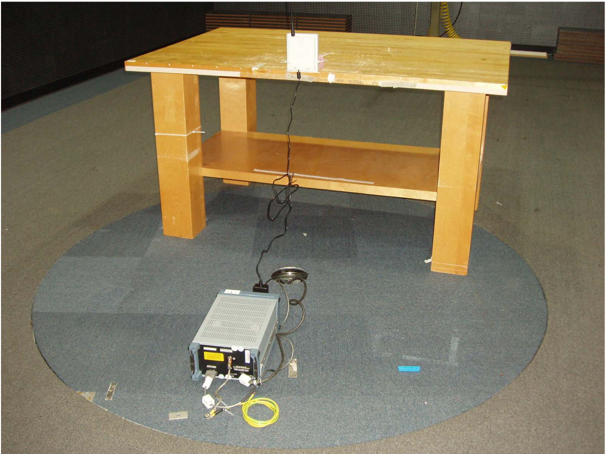
Photo 6 – AC Mains Conducted Emissions Test Set-up
