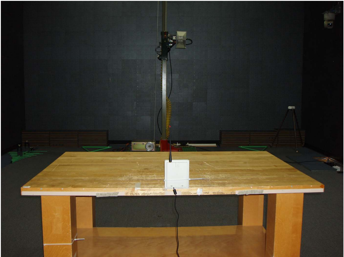
Photo 5.5-3 - Rear View of the Radiated Emissions Test Set-up above 1 GHz
