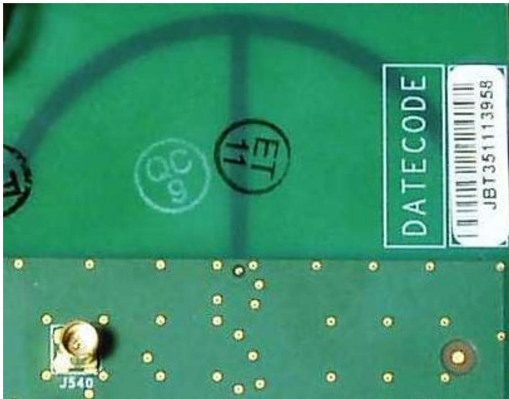
The radio board includes an integrated Printed Circuit Board (PCB) trace antenna with a nominal gain of -2.0 dBi.
