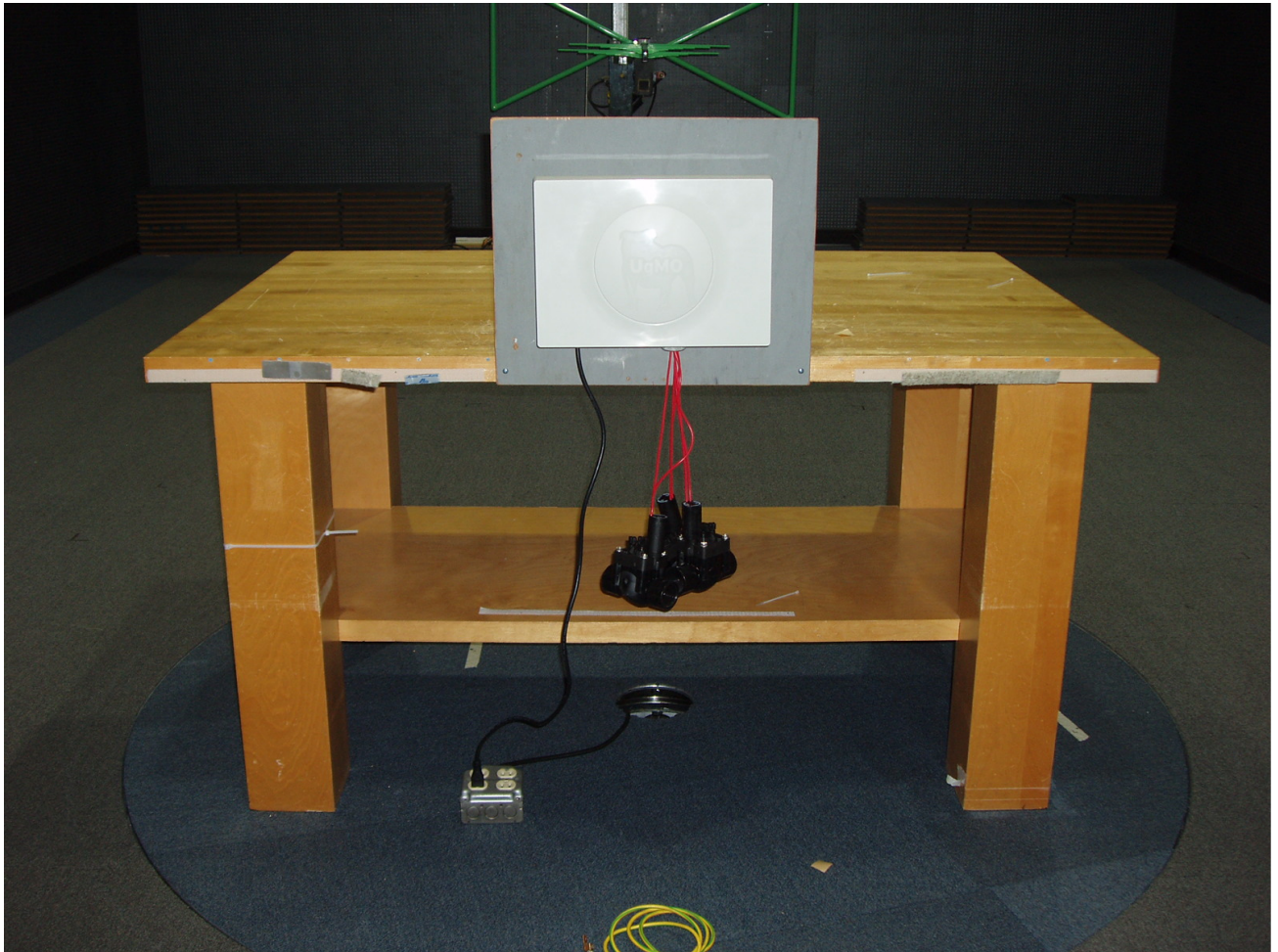
Photo 2 – Rear View of the Radiated Emissions Test Set-up
