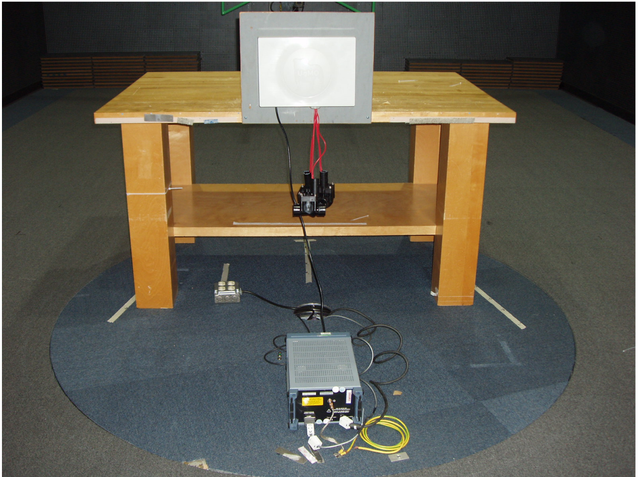
Photo 4 – AC Mains Port Conducted Test Set-up
