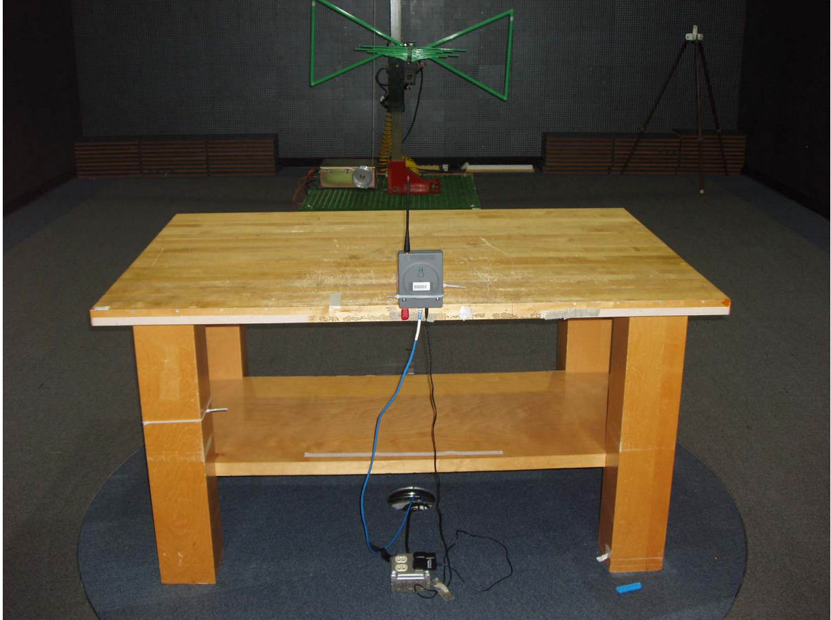
Photo 5.5-2 - Rear View of the Radiated Emissions Test Set-up 30 – 1000 MHz
