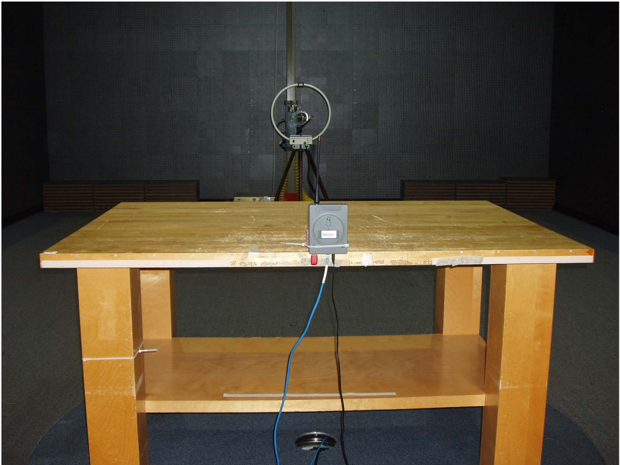
Photo 5.5-4 - Rear View of the Radiated Emissions Test Set-up with the Loop Antenna
