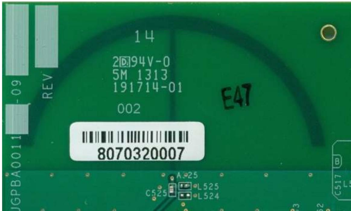
The radio board includes an integrated Printed Circuit Board (PCB) trace antenna with a nominal gain of -2.0 dBi.
