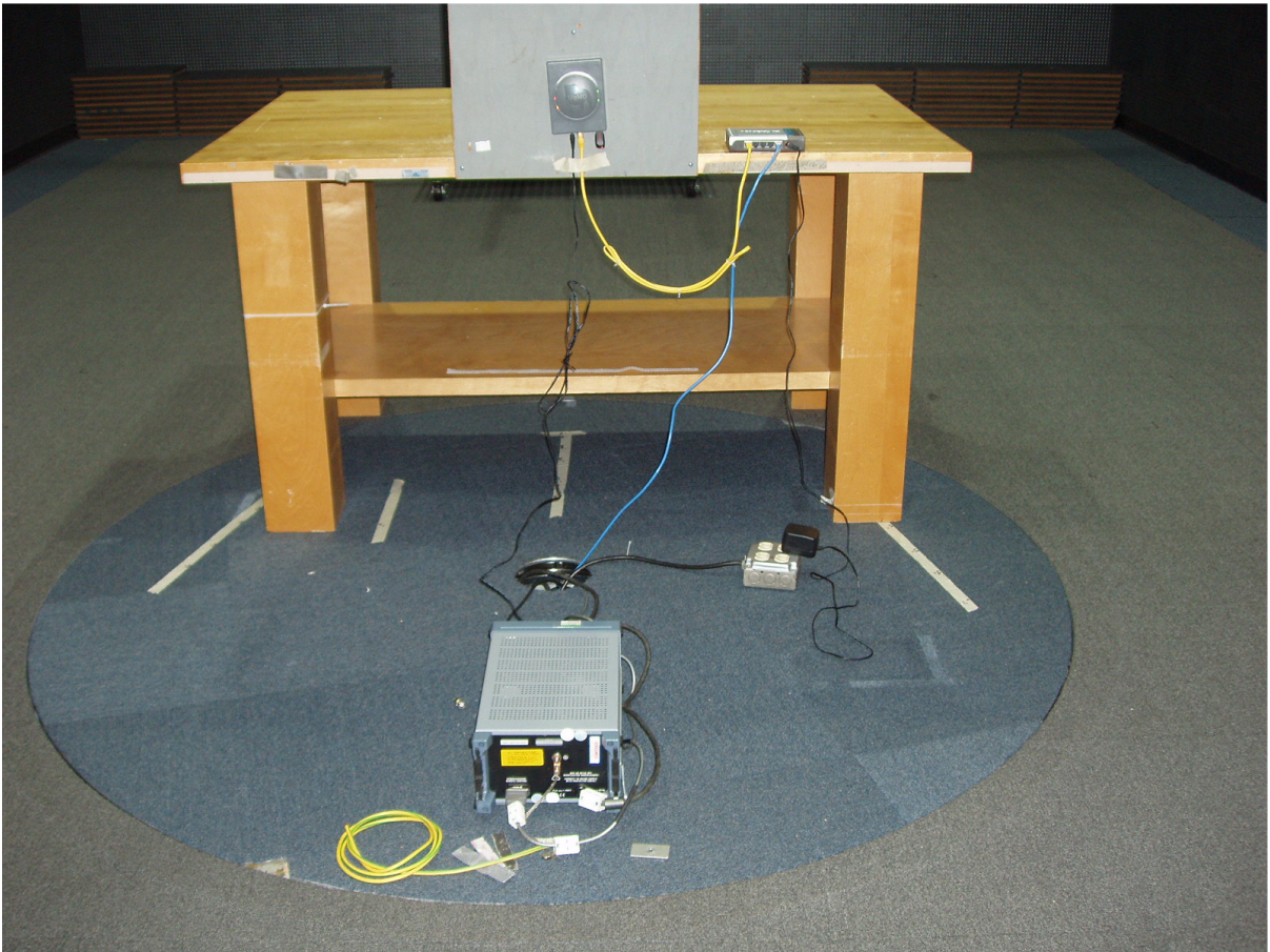
Photo 5 – AC Mains Conducted Emissions Test Set-up
