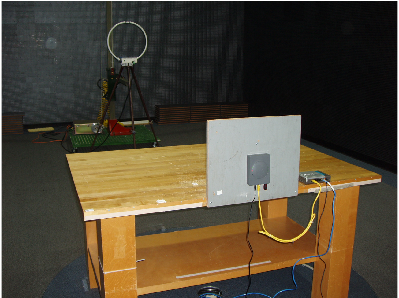
Photo 5.5-3 - Rear View of the Radiated Emissions Test Set-up with Loop Antenna
