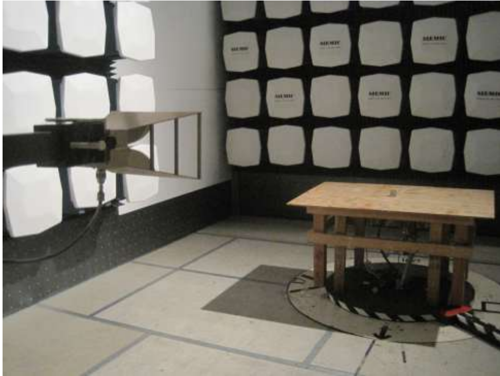
Radiated Emission (>1GHz) Setup Front View
