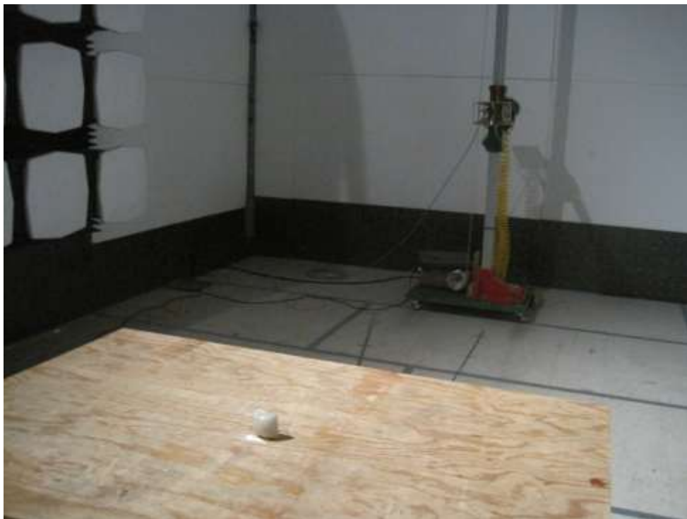
Radiated Emission (>1GHz) Setup Rear View
