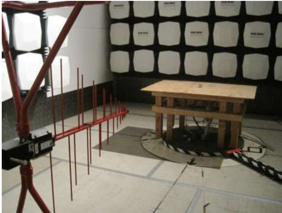
Radiated Emission Front View (30MHz-1GHz)
