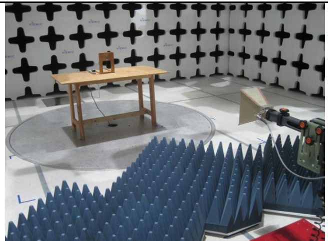
Test setup at 3 meter distance (>1GHz) - Rear
