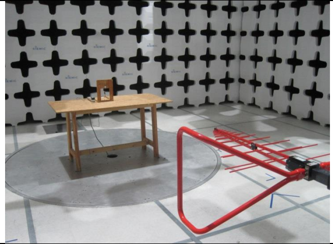
Test setup at 3 meter distance (<1GHz) - Rear
