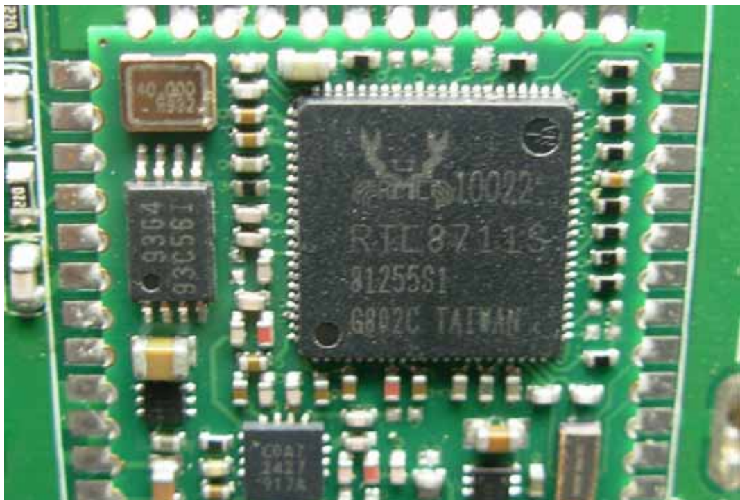
FIGURE 10 10.1 INCH DIGITAL PHOTO FRAME (M/N: LP-101WT) CHIP & CRYSTAL ON RF MODULE
