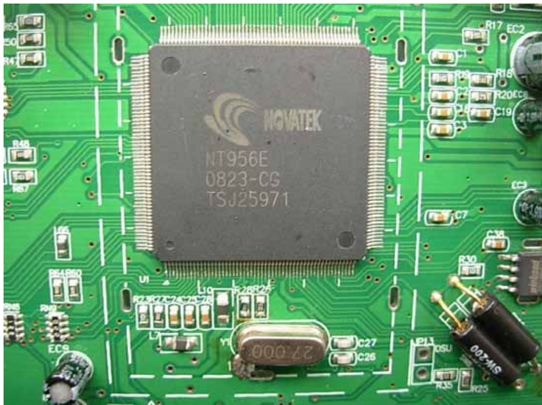
FIGURE 8 10.1 INCH DIGITAL PHOTO FRAME (M/N: LP-101WT) CHIP & CRYSTAL ON MAIN BOARD
