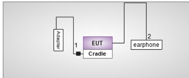
1. 1.1m non-shielded cable with one core
