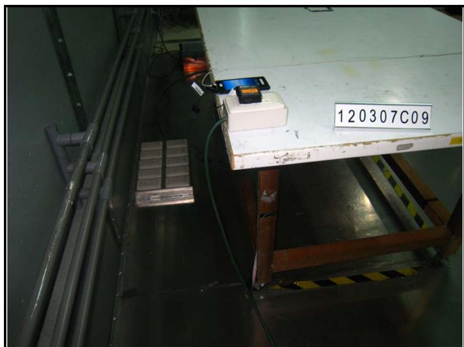
RADIATED EMISSION TEST (X-Axis)
