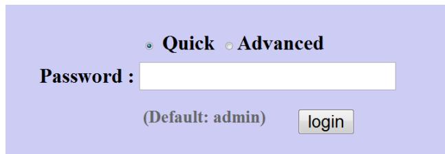
Select the '**Quick**' option to quickly configure the router's basic settings, such as setting the Dial code, APN and wireless security.
