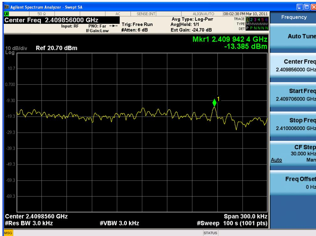
**Power Spectral Density (802.11n-CH 6) – 20 MHz**
