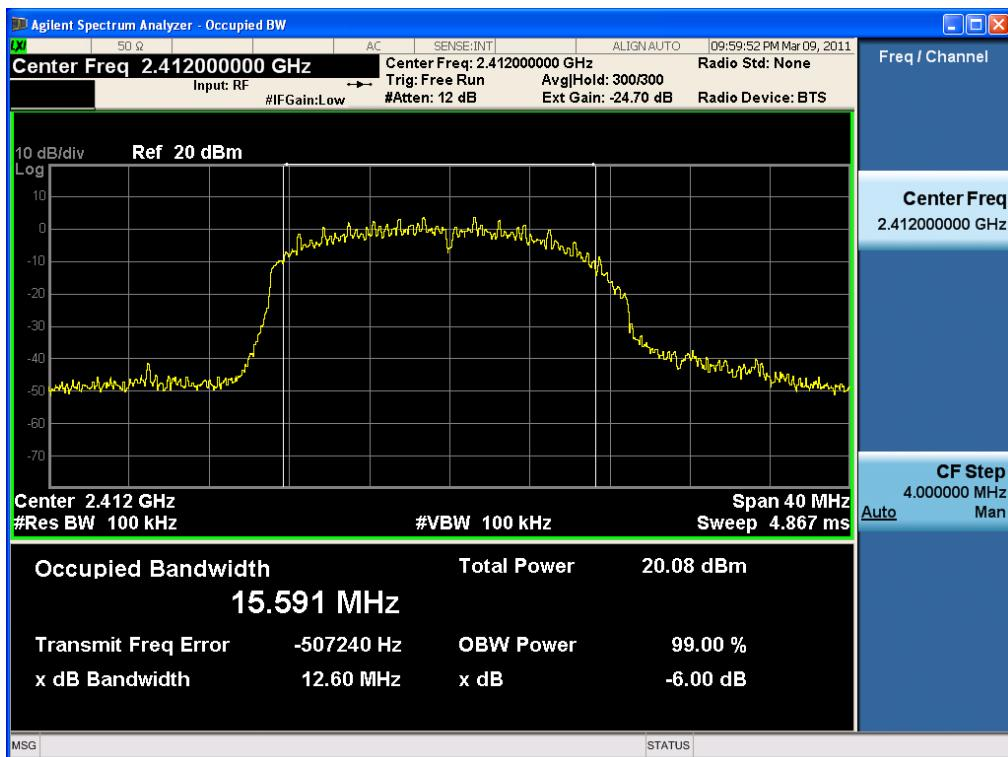
**6dB Bandwidth plot (802.11n-CH 6) – 20 MHz**
