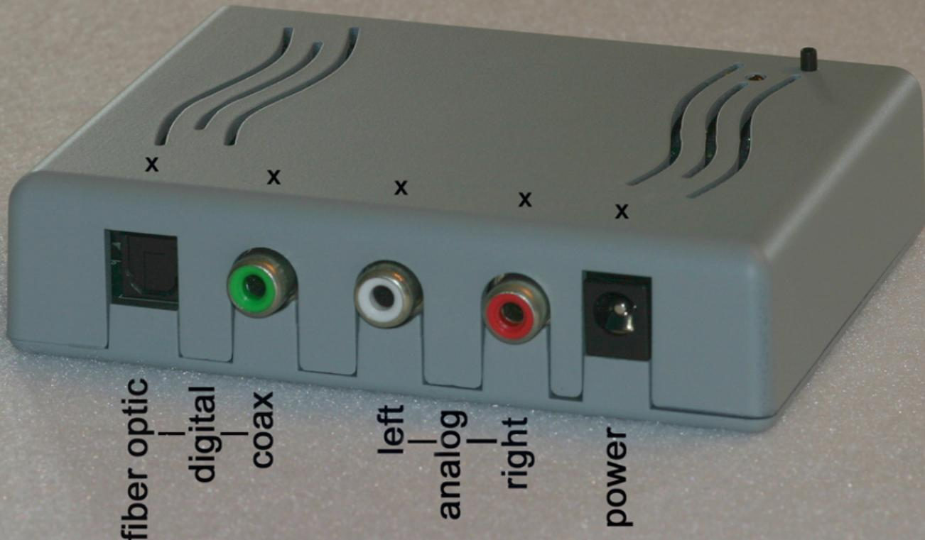
The connector names will be molded into the housing where you see the x's
