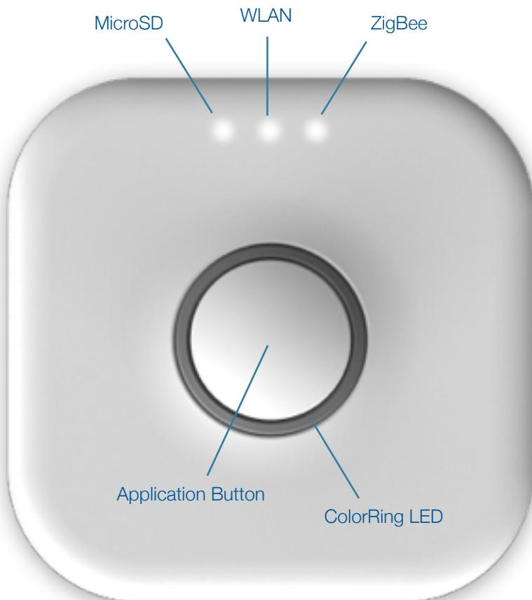
The RSG-3000 Wireless Smart Gateway has the status LEDs shown in the above figure.
