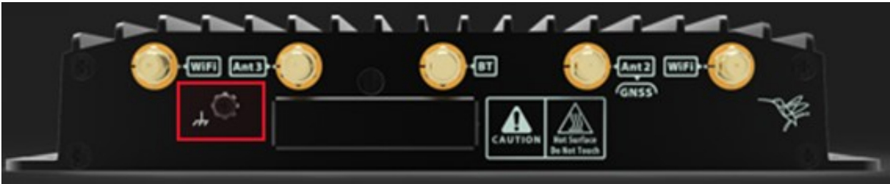
Fig. 13: Rear view, Protective Earth connection
