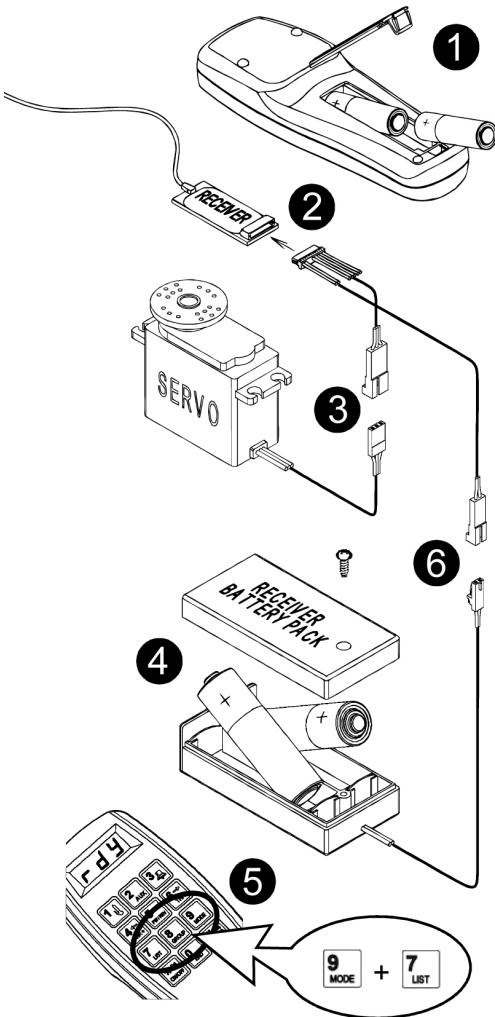
1. Install two AA Batteries in Transmitter. *(display will show that System is Ready)*
