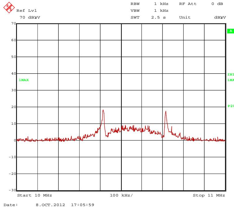
The centre frequency of the transmitter was found at 10.57 MHz. It had to be measured on the outdoor test site. The results are shown in clause 5.1.2.2.
